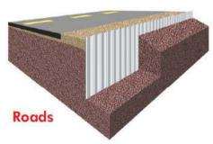
Tidewall can be used in several ways in road construction. First, for roads that are built across a slope, Tidewall has been used as a retaining wall to allow construction of a shoulder, and to diminish the gravitational stress on the roadbed. Second, it can be used as a cut-off or seepage wall to keep subterranean water away from bridge abutments and road supports.
